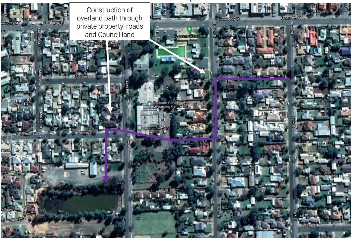
Figure 8-5 Key Features of Mitigation Option P9
